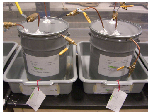
A: Pipe water sampling and replenishing tubing B: Drum solution replenishing tubing C: Steel restraining strap D: Ductile iron pipe joint E: Gasket
